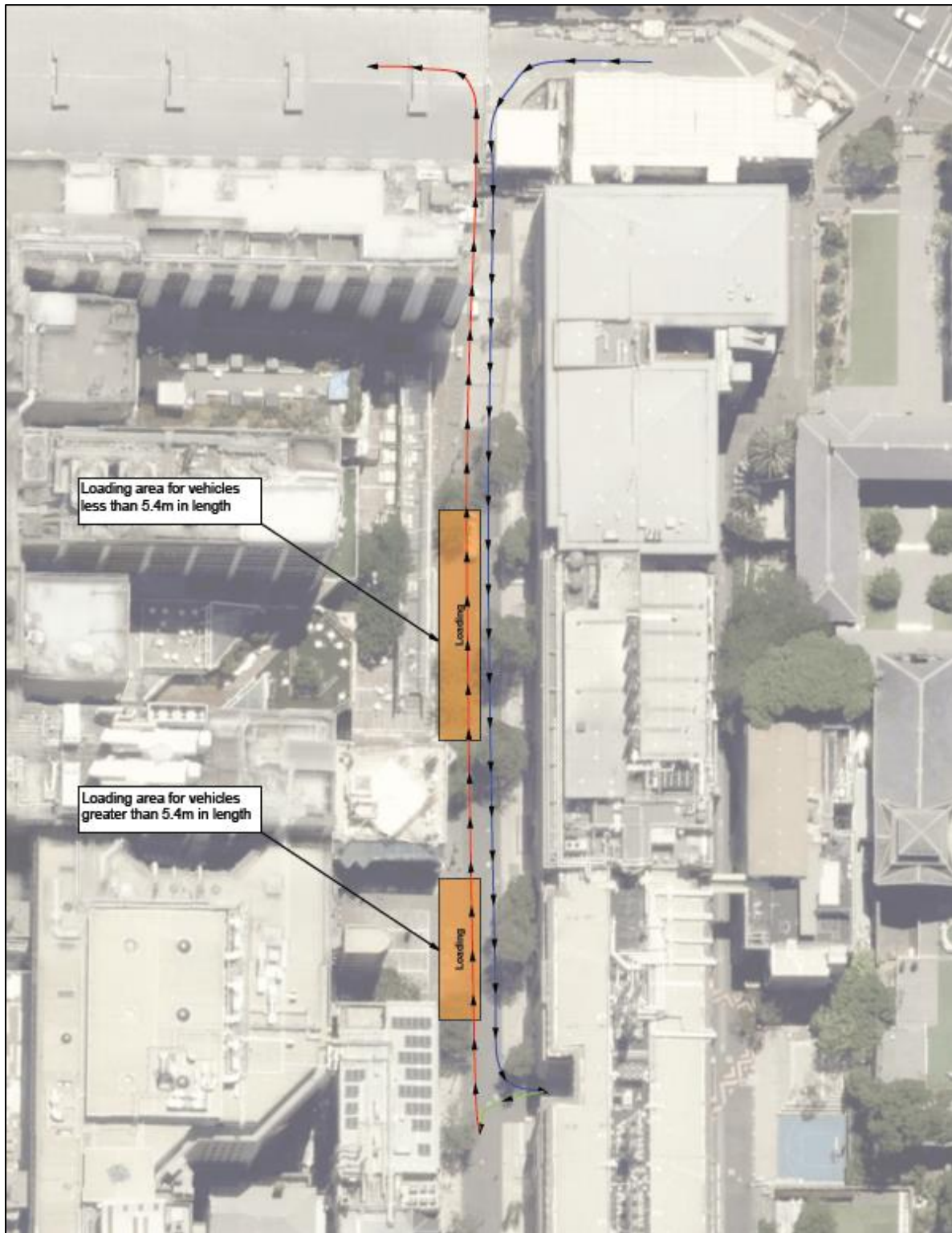
Figure 2.6: Future Access Arrangements – via Franklin Street
