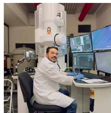
Conducting a HRTEM sample measurement at RMMF
