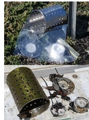
Passive samplers and housing before and after deployment
